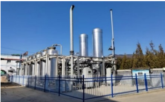
图11 低浓度煤层气变压吸附提浓工业化示范装置 Fig.11 The industrial demonstration plant for low-concentration coalbed methane enrichment by pressure swing adsorption
